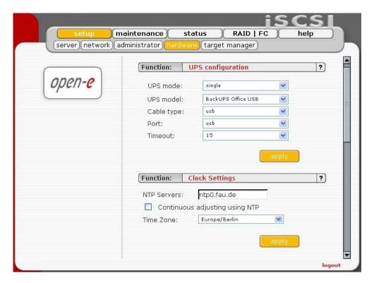
In the settings you can select the UPS model, cable type, connection port and the length of the time out. The time-out defines the time between a power failure and the moment the system will shut down. UPS support in mode "Single" means that Open-E iSCSI is the only system attached to this UPS and that there is no action necessary to do remote shutdown for other systems in the network.
